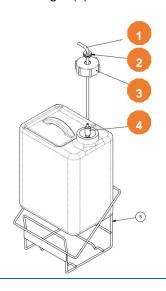
4. Ensuring the tube is fed so that there is excess tube at the bottom of the bottle, screw on the lid.
